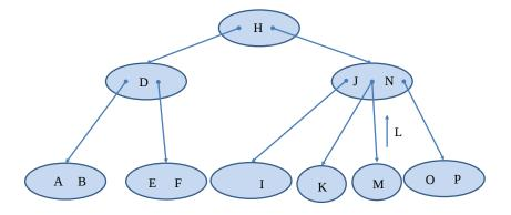
The node is split in two and Lis passed to the parent node
